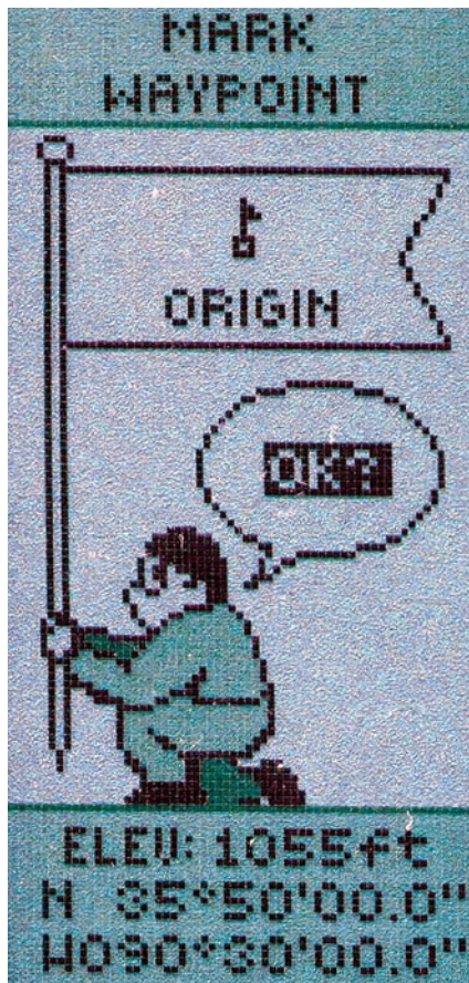
Figure 1 Create a waypoint with the latitude and longitude of the State Plane Coordinate Grid Origin.
