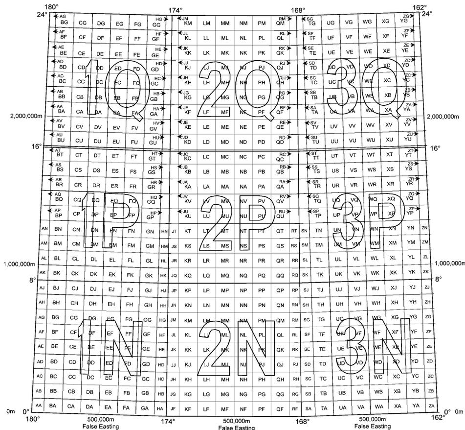
Figure 2 Basic Plan of the 100,000-meter Square Identification of the USNG
