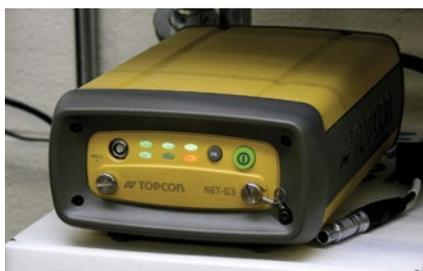
At the heart of it all, Topcon's NET-G3 offers capability to track GPS, GLONASS and Galileo satellites.
