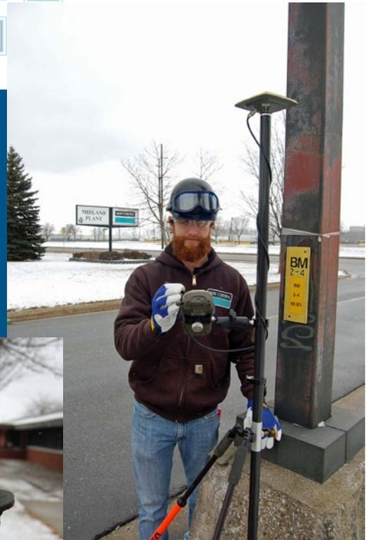
**Left:** Topcon’s GRS-1, working in conjunction with Michigan DOTs CORS network, provided the survey-grade RTK accuracy needed for the GIS project.
