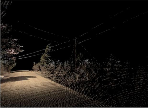
Georeferenced 3D LiDAR point cloud data viewed in Spatial Factory software.
