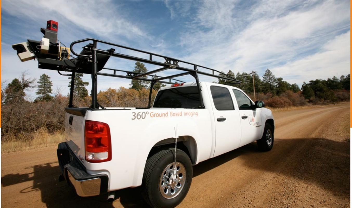
GeoNav's vehicle mounted 3D mobile mapping IP-S2 system maps rural America.
