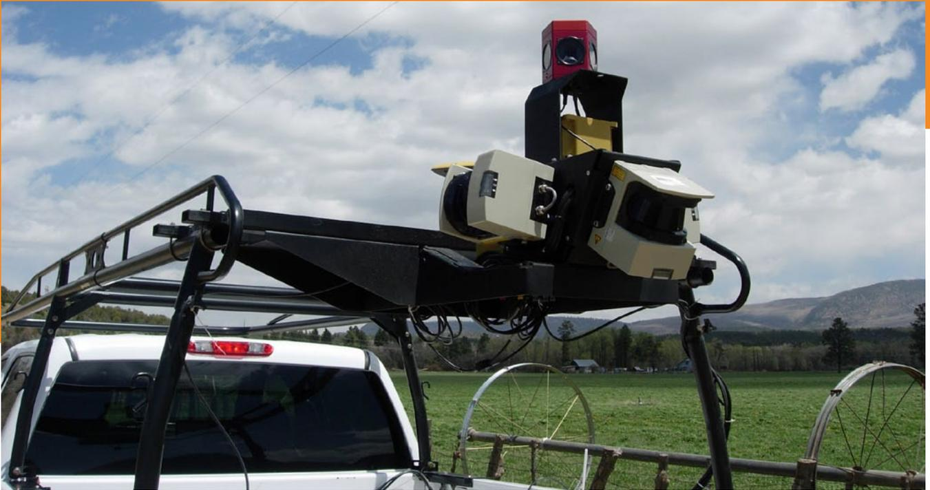
A close-up view of the IP-S2 3D mobile mapping system shows integrated 360-degree camera, laser scanners, GPS tracking and IMU components.
