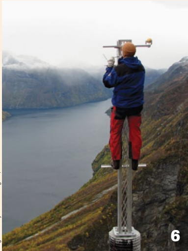
Atle Gerhardsen of Norwegian geo-monitoring company Cautus Geo attaches a prism, collocated with a GNS antenna at one of many monitoring masts at the site of their Åknes fjord monitoring project.
