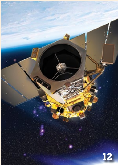
An artist's conception emulates the high-resolution GeoEye-1 satellite orbit. The satellite flies 423 miles (680 km) above the earth at an average speed of 17,500 mph (4 miles per second).
