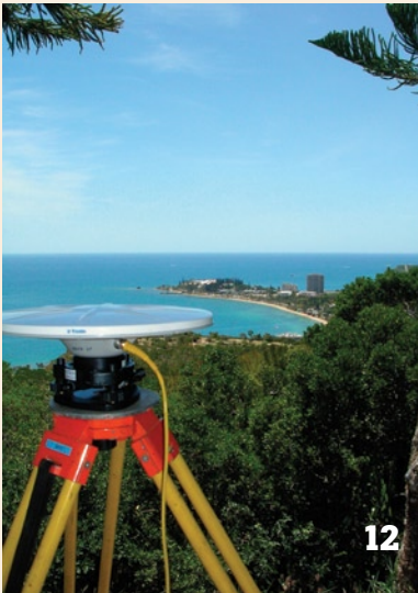
A Trimble Zephyr Geodetic Antenna [ZGA] is set up as a temporary base station at Ouen-Toro (Nouméa) in New Caledonia.
