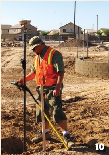
At Woodcrest Village in Gilbert, Arizona, Atwell-Hicks Party Chief Josh Lemons uses a Trimble R8 to check in to a control point established using the AZGPS VRS network.
