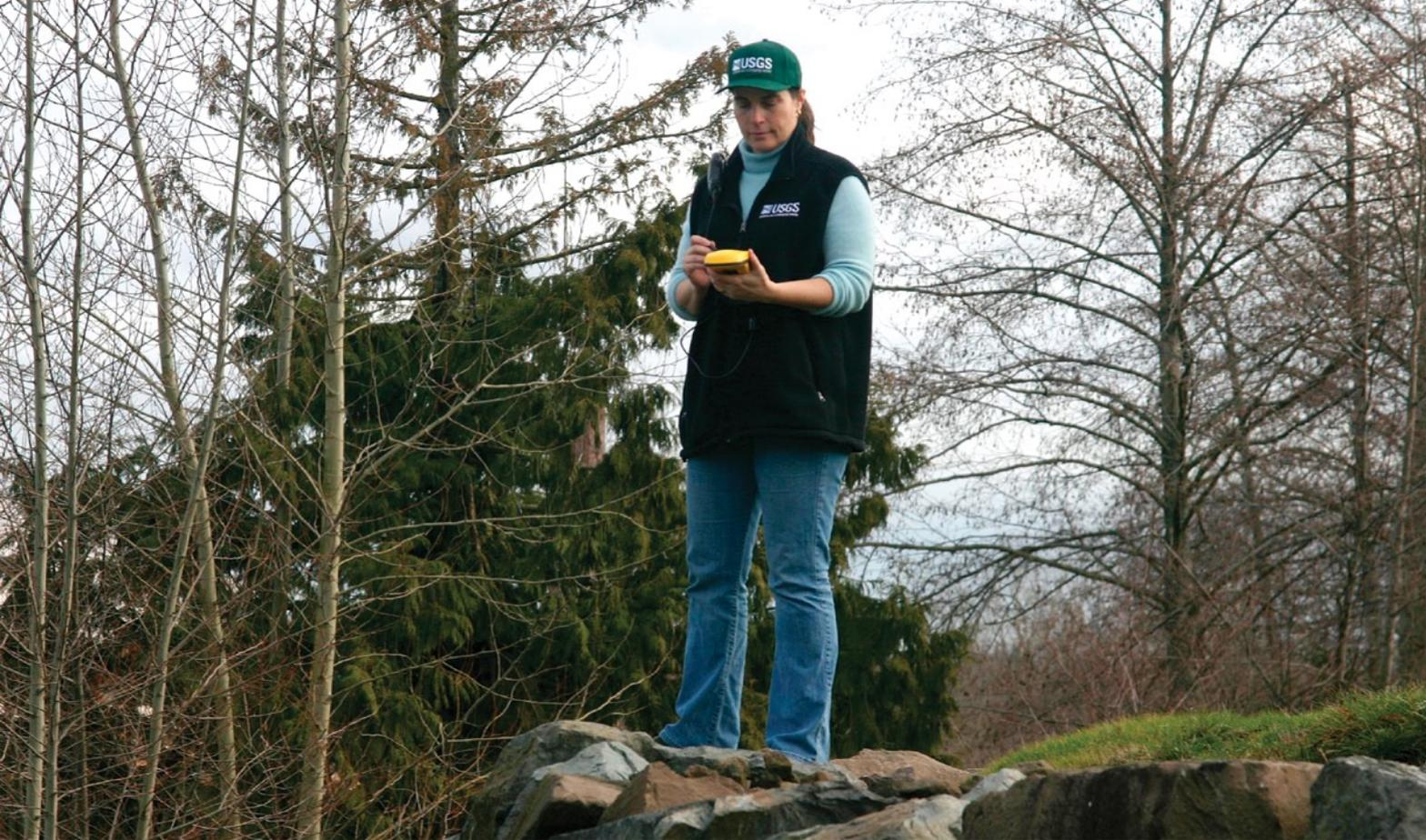
Vivian Queija evaluates canopy conditions for a shoreline mapping project. Later Vivian would attach an external antenna on an extended rod in wooded areas of the project, and then an external dual frequency receiver for higher-precision vertical observations on shoreline bulkheads and drainage outfalls.
