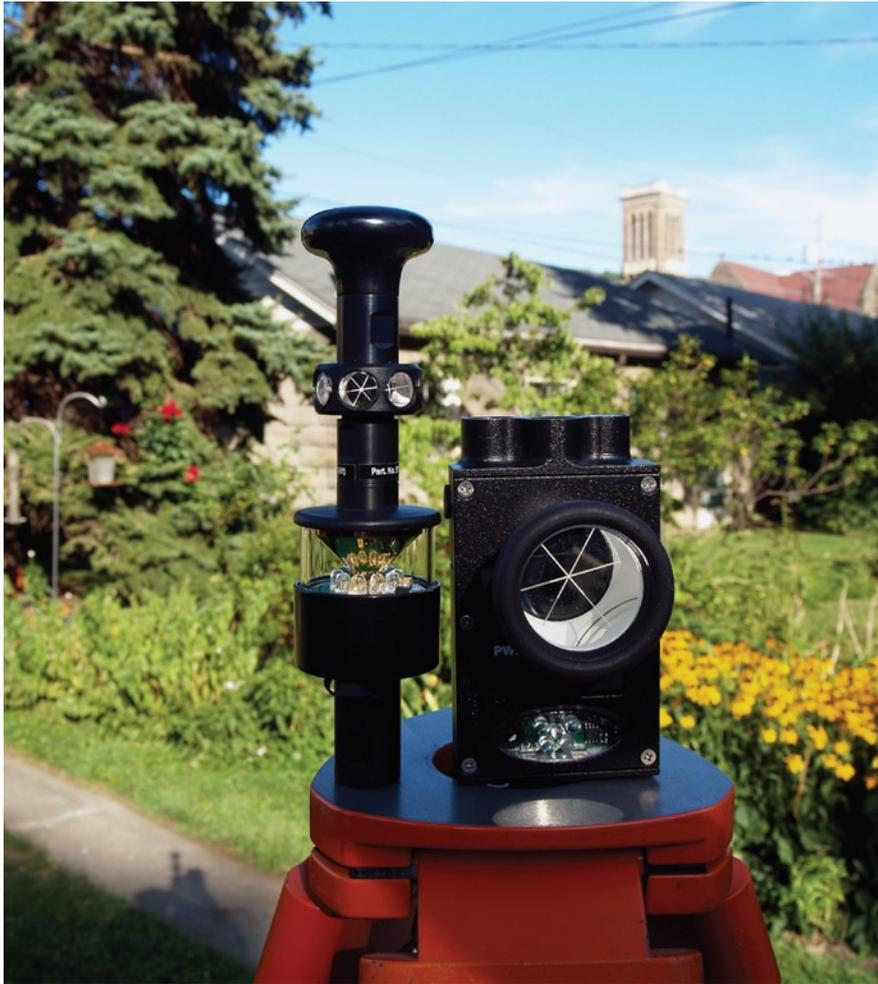
360° prism/diodes for use at the prism pole, (left) and RMT 602 for traversing, (right).
