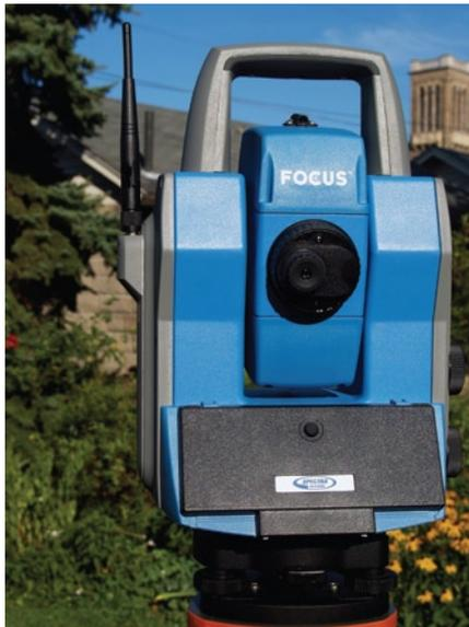
Focus 10 with cover in place of key pad for controlling operations from the prism pole.
