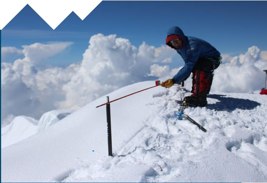
Horner with two GPS antennas. In the foreground is a survey monument stuck in the snow in 1989 by Jeff Yates during his original GPS survey; it is not anchored in the ground as required for an official NGS monument.
