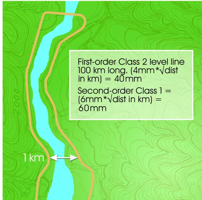
**Figure 2** Example of accumulated errors from differential leveling over long distances
