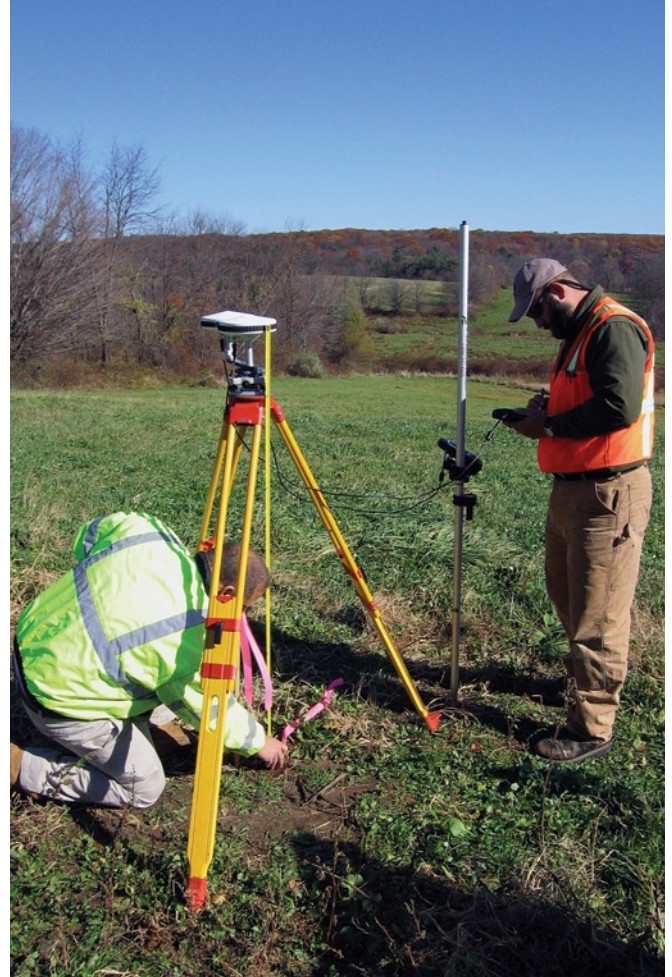
Laferriere measures the height to the antenna during initialization setup.
