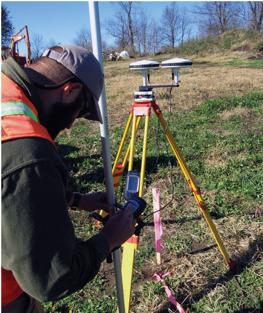
Assistant Chet Kasper initializes the ProMark3 rover with the aid of an initializing bar consisting of the two antennae 20 cm apart.
