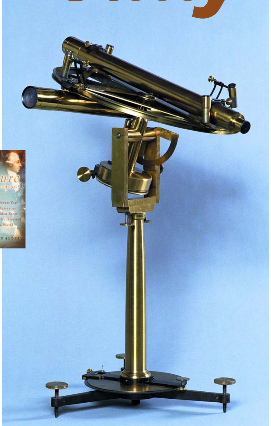
Repetition circle built by Etienne Lenoir in Paris around 1800. This instrument is nearly identical to the ones Méchain and Delambre used during the French meridian expedition (1791-1798). It was used in the first triangulation of the Netherlands (1802-1811). The Dutch network was connected in Dunkerque with the French meridian triangulation, thereby providing a link between the French and Danish triangulation networks. Photograph courtesy Technology Museum Delft University, The Netherlands.
