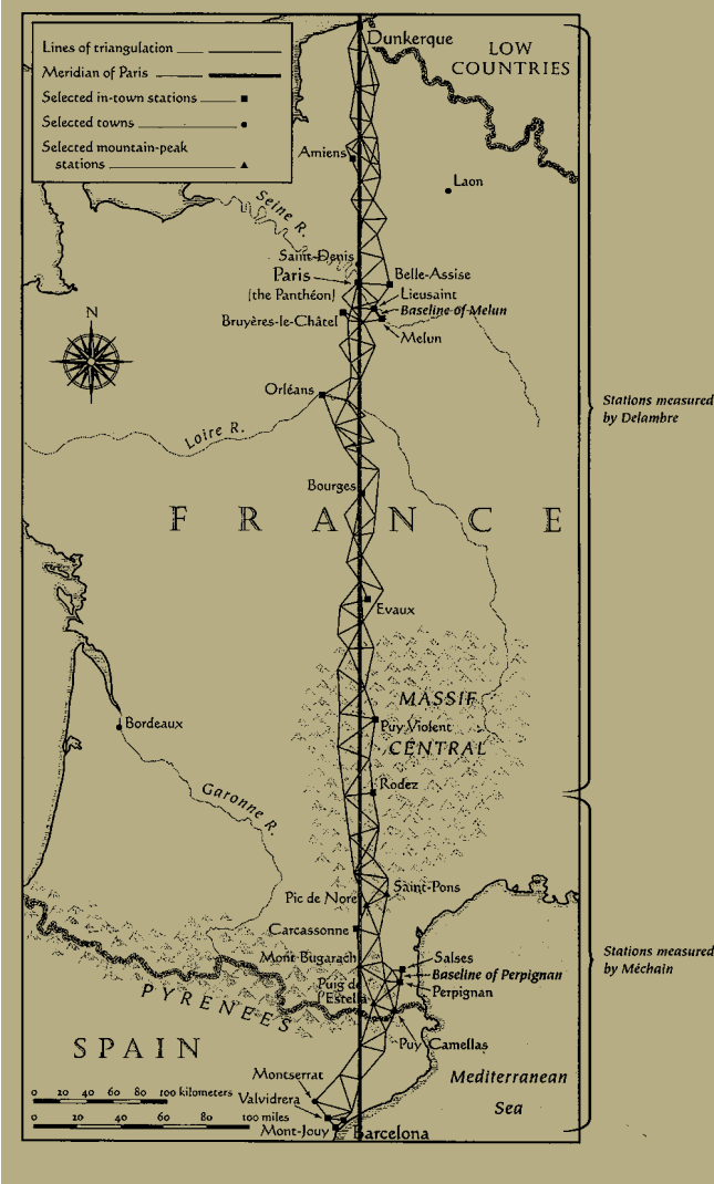
This map, adopted from The Measure of All Things , is from an original map in Paris. It shows the original arc of triangulation from Barcelona to Dunkirk as performed by Méchain and Delambre.
