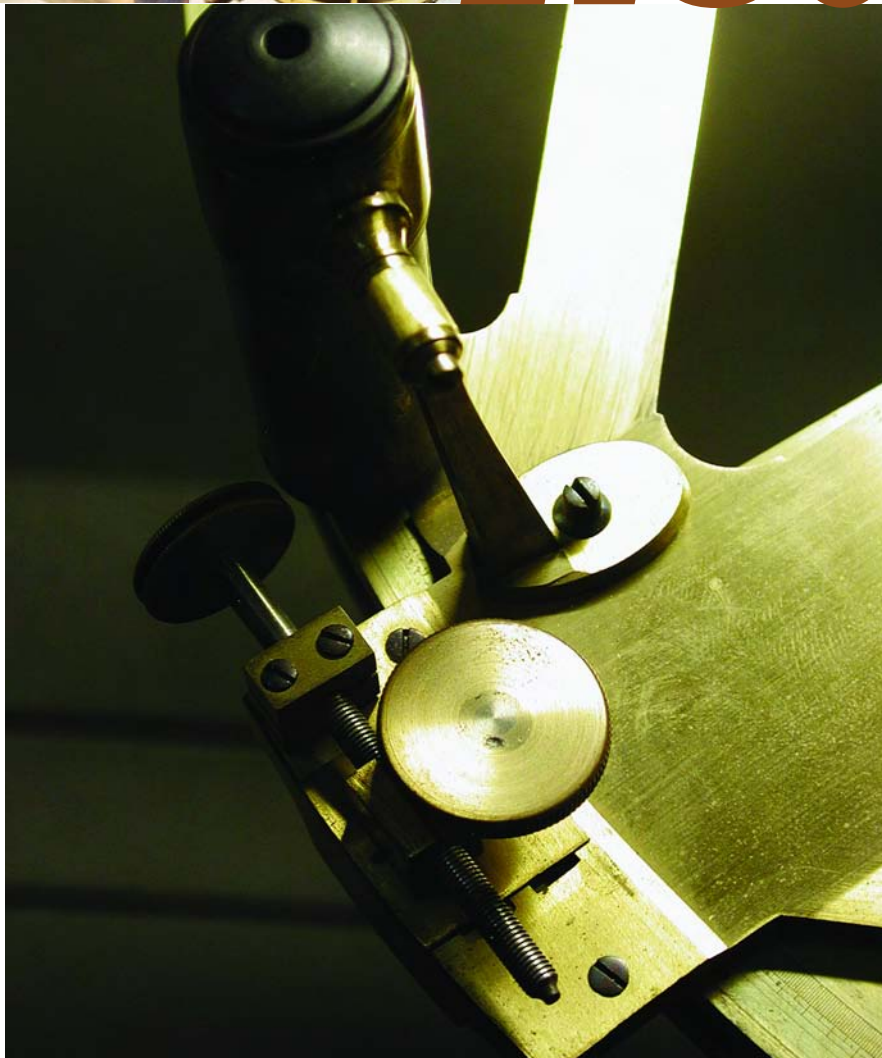
Constructional details of the lower left corner of square frame that supports the upper telescope include a cramp (screw), a setting screw and an eye piece for reading the circle.
