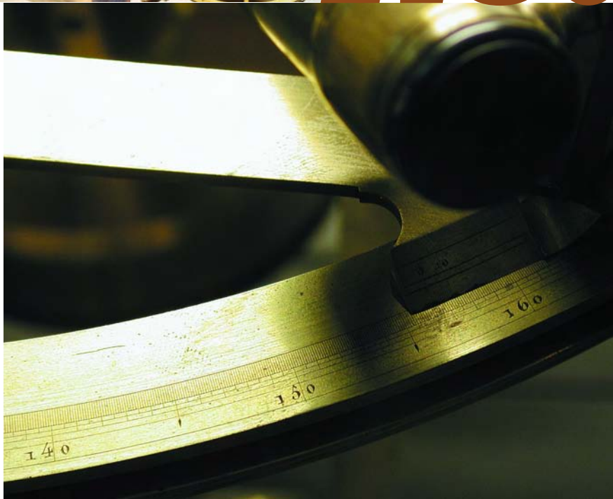
Part of the circle between 140 and 160 grads (gon) showing the subdivision of one-tenth. The vernier, which is fixed to the square alidade holding the upper telescope, allows reading the circle with a precision of one-hundredth of a grad (gon).
