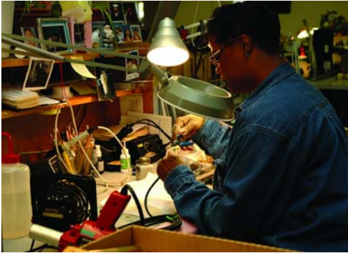
Top left & right: Locator assembly takes place at about a dozen small work stations, all packed with hundreds of small parts and tools.
