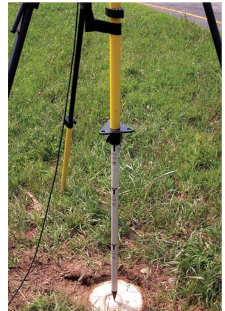
**Quality control: Fixed height tripods should be employed when using GPS to better insure quality.**
