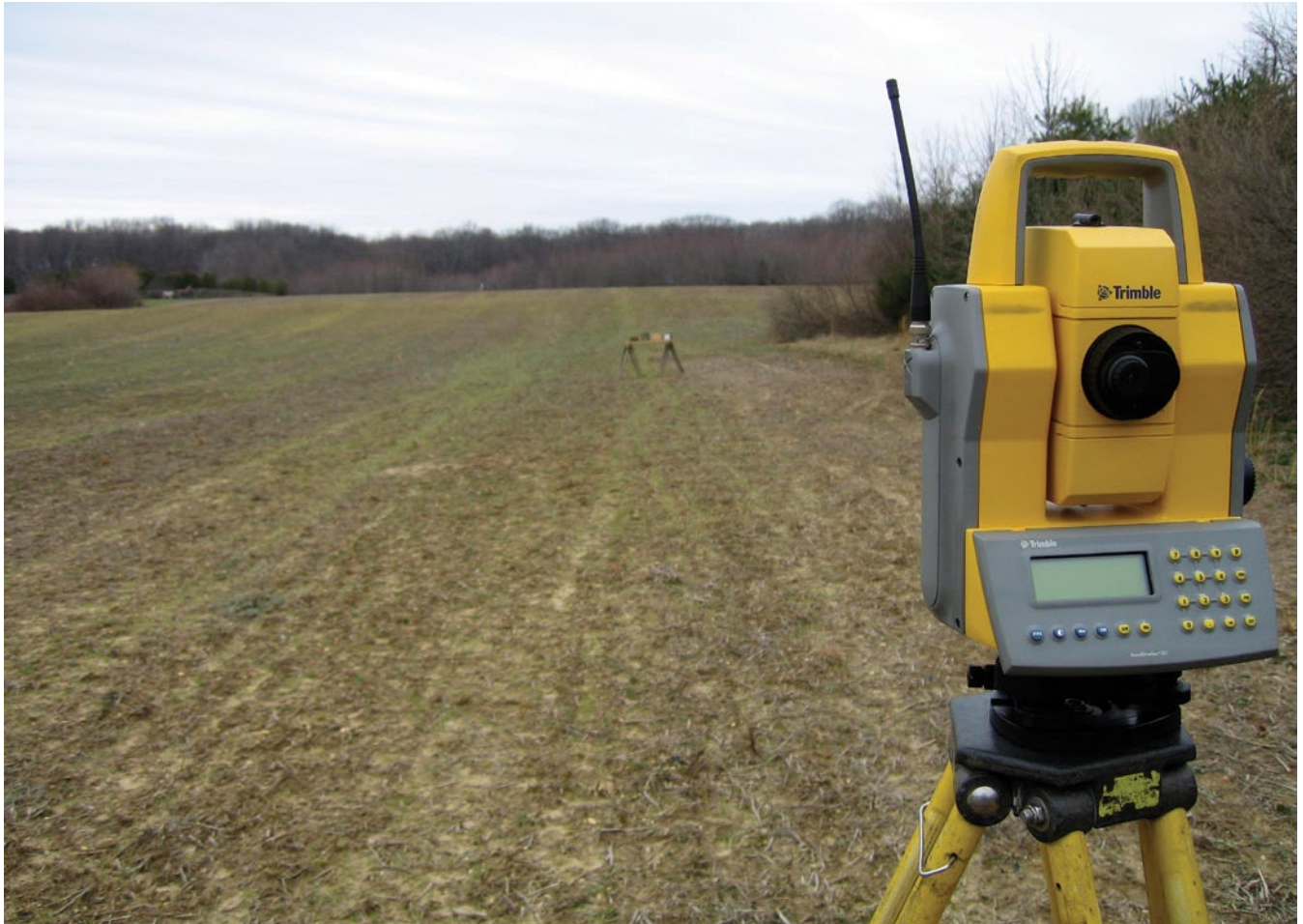
Trimble Robotic Total Station 5600 SeriesDR200+ at staging area with material samples in background.
