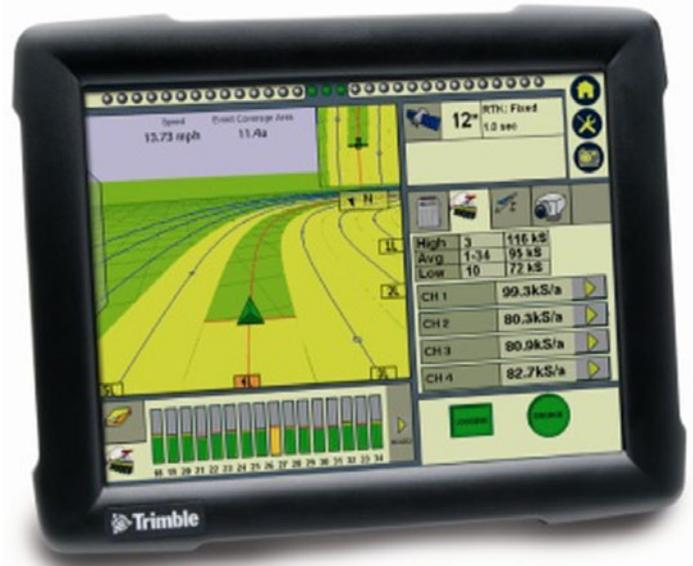
Figure 5 Typical in-cab AMG controller
