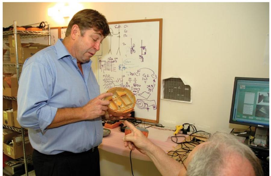
Vancans discusses the critical issue of component placement and demonstrates how one screw can cause parts to interfere with each other.
