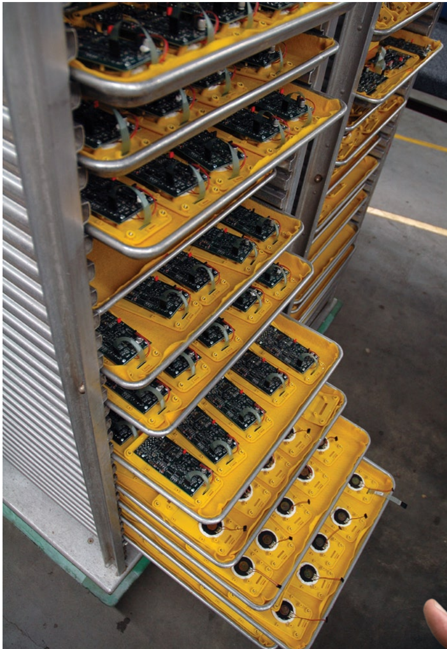
This old baking tray cart has been converted to a parts tray cart.
