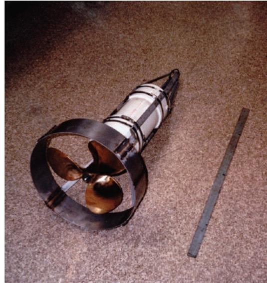
The towed generator was used to charge batteries on the run, thereby eliminating interruptions for battery service.
