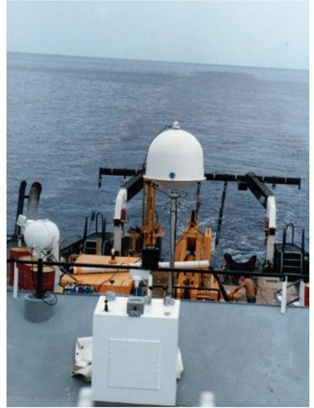
View of the rear deck showing STARFIX antennae mounted amidship.
