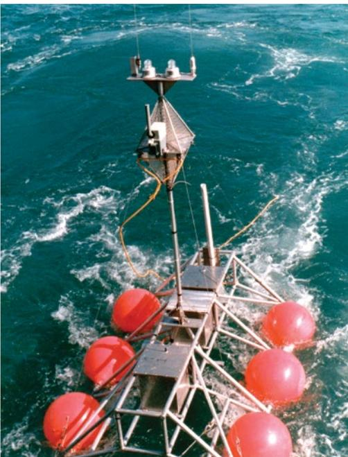
Seismic array tail buoy sporting bright floats, RADAR reflector, flashing lights, LORAN, radio, batteries and probably towing a generator.
