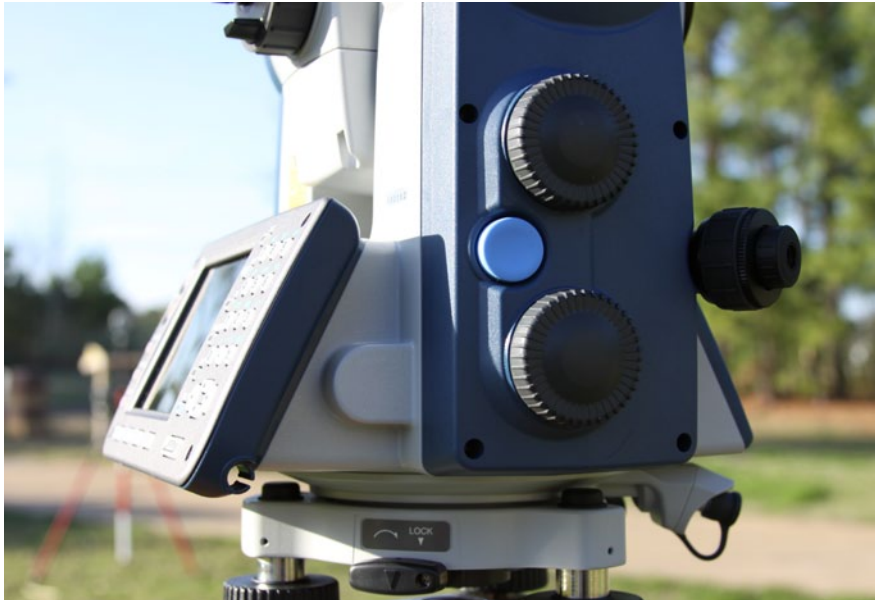
The SRX proved to be an ergonomically friendly instrument while operated conventionally. Here the two jog/shuttle motion knobs can be seen as well as the thumb initiated measurement trigger between them.
