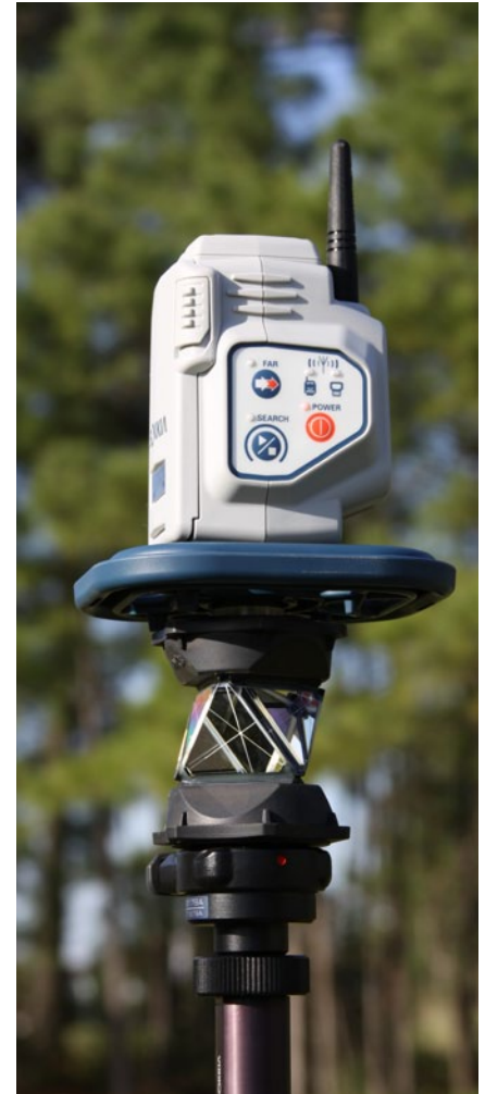
The ATP1 360° prism provides practically no distortion due to parallax and is secured by a quick release attachment. Atop the prism is the combined RC-PR4, the integrated Bluetooth radio transceiver and infrared dog whistle, used to communicate with the SRX or redirect it should it lose lock.
