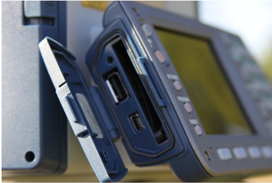
The SRX neatly conceals the Compact Flash (Type II) Slot and USB client (for PC hookup) and USB host (for USB memory).
