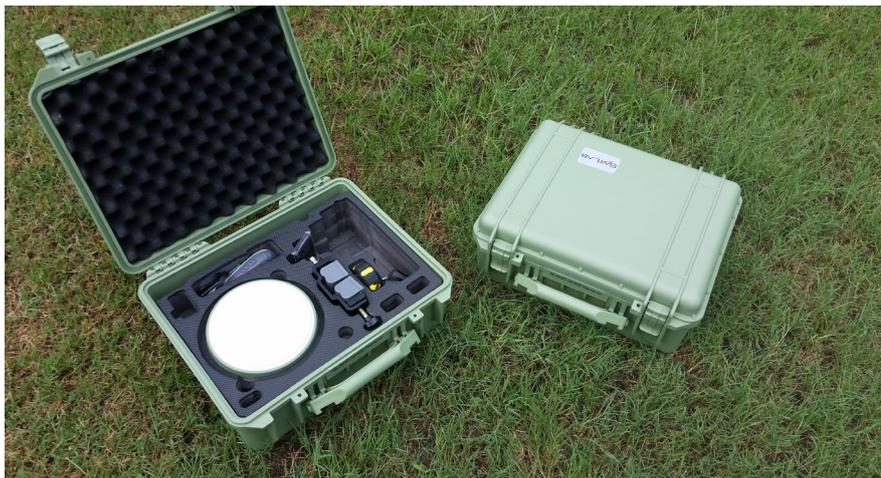
The SL600 system comes packaged in well-constructed hard-shell cases suitable for carrying everything needed for RTK surveying except for the rover pole and tripod.
