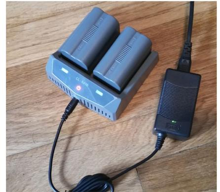
Two dual bay chargers are provided with the system allowing for four batteries to be charged at a time. Once charged, the system is ready for up to 16 hours of operation when operated as a base or 24 hours as a rover.
