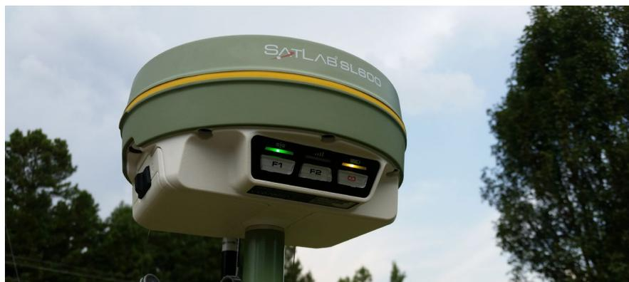
The SL600 receivers have a durable feel. The LED panel gives the user the receiver's status at a glance and provides three buttons for controlling commonly accessed features.
