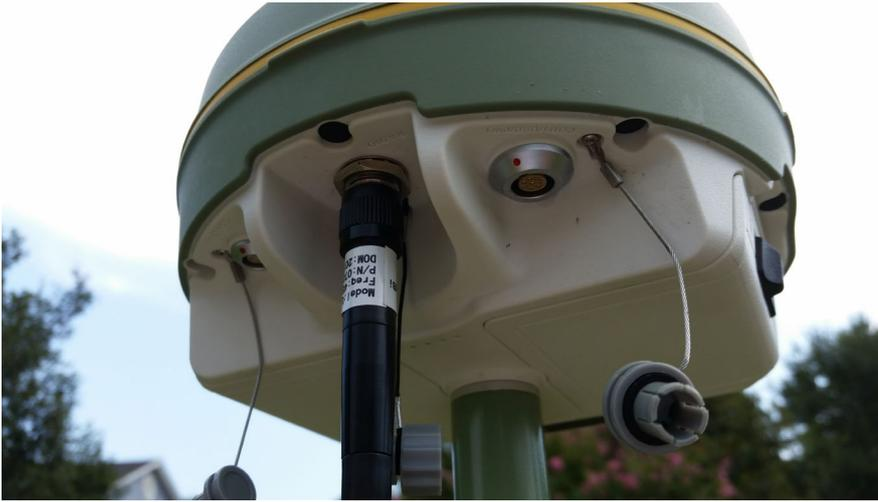
The placement of the UHF antenna in a recess on the bottom of the receiver provides some protection from incidental contact which commonly occurs during field use.
