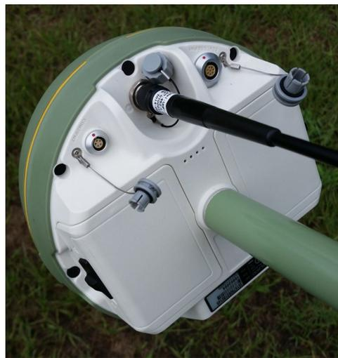
The battery latches proved easy to manipulate and secure. The compartments house the batteries as well as the SIM card and MicroSD card slots. The two standard LEMO ports provide access serial connections to external controllers and radio modems.
