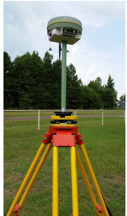
The SL600 receivers can be configured as a base (reference station) or rover. Here the SL600 is setup as a reference station.
