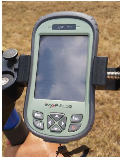
The SL-55 Data Collector with Carlson Software SurvCE or MicroSurvey Field Genius controls the SL600 system.
