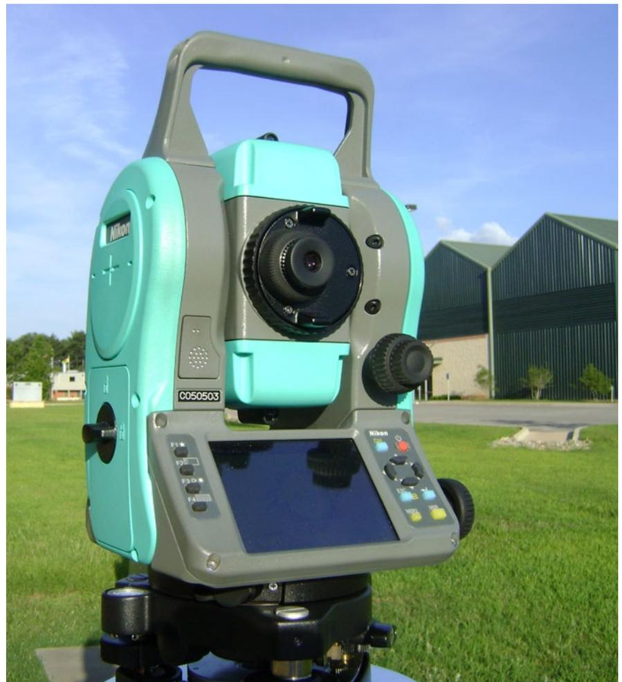
**The Nikon Nivo C offers sophisticated data collection in a Windows CE environment, a large touch screen, reflectorless distance measurement with a respectable range, and two onboard hot-swappable batteries, all in a light, compact package.**
