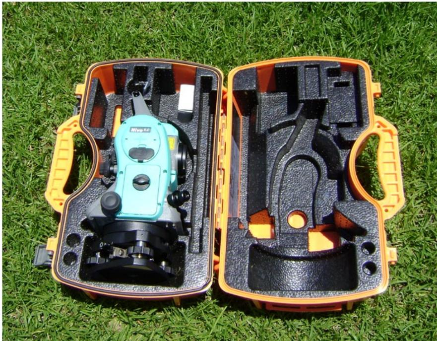
The Nivo C instrument station is complete with this small box and a tripod. With Survey Pro software on board, it presses the question, “Why am I still toting an external data collector?”
