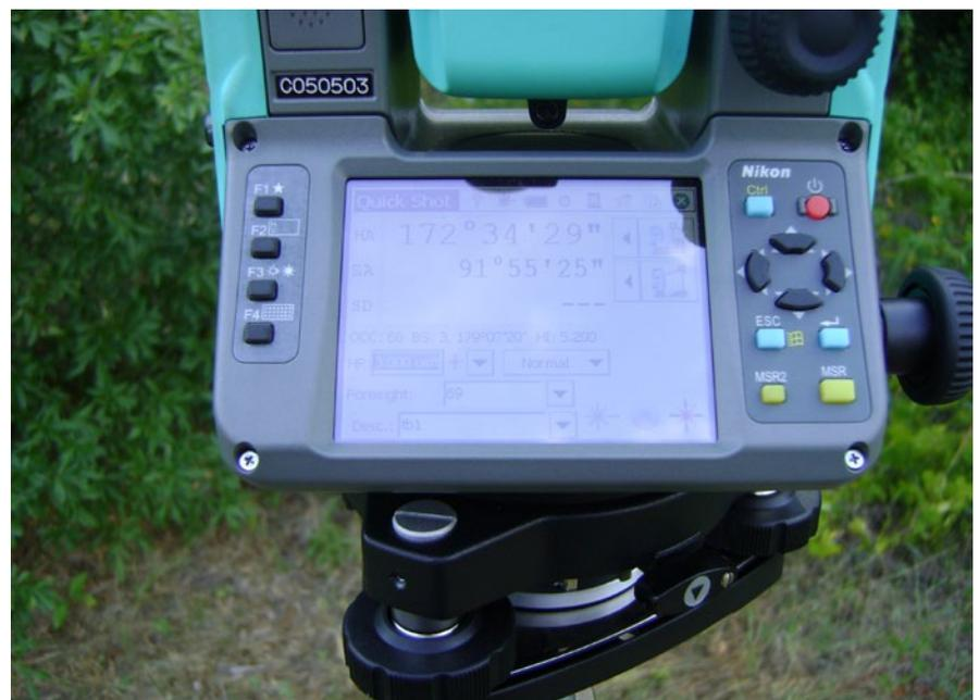
The screen on the Nivo C is generously proportioned and bright even in the outdoors. With a little practice you can press the yellow MSR button with your thumb and adjust the knob with your fingers while peering through the optics.
