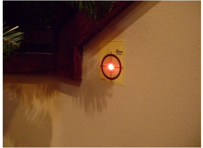
The laser dot is useful for determining where the instrument is pointed, particularly when the streaming video image becomes more difficult to use. In most interior spaces the dot will be easily visible. Seen here, the laser is collimated on a supplied paper target for a resection.
