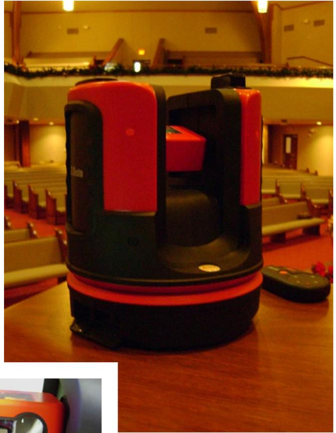
Because of the Disto 3D's design, I was able to set it up on this organ and measure most of the interior of this auditorium. Because it has no scope, I did not need to worry about how I would move around it.
