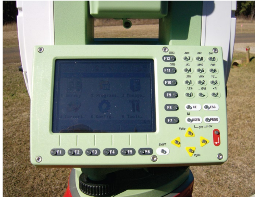
The TPS1200+ can be operated using onboard software that is identical to the software found on the RX1250.
