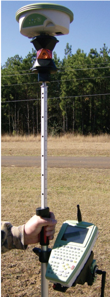
Leica ATX1230 SmartAntenna, 360° prism and RX1250 data collector combine to make the SmartPole.
