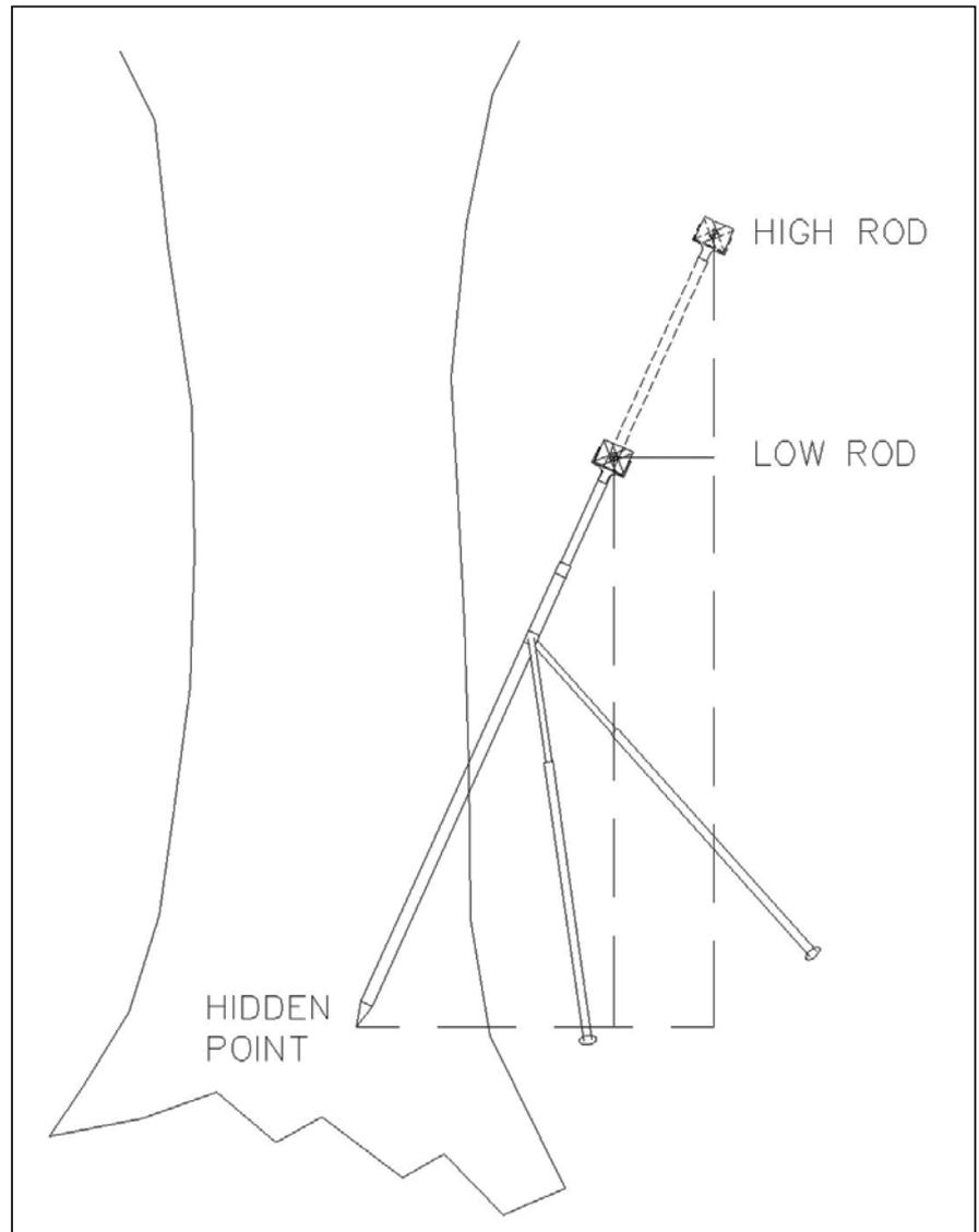
This schematic shows the basic principle of similar triangles, which makes this method work. Notice the right triangle being formed by the hidden point, the low prism and the offset at the ground, as well as the the triangle formed by the hidden point, the high prism and the offset at the ground. These two triangles are said to be similar (the angles are the same). This is the foundation of the Hidden Point Offset.
