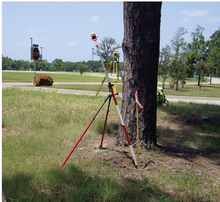
Setting the pole up, your rodman must be diligent to firmly place the bipod legs in the ground and do everything possible to keep the pole point from slipping. The alignment of the pole must remain the same as the two shots are being made or the method will yield inaccurate results.
