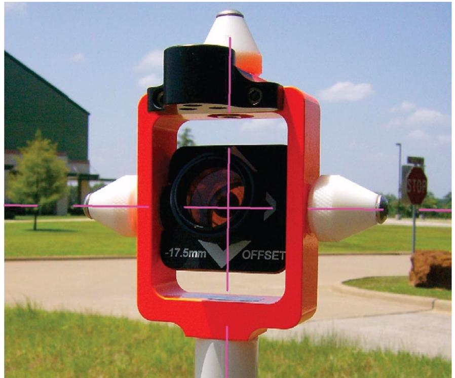
As you can see in this photo, the reflection of the camera lens is at the center of the true nodal prism. Overlaying the horizontal axis and vertical axis, you will find that the apex, or nodal point of the prism, is precisely coincident with the intersection of the axis lines even though the prism is not directed toward the camera.
