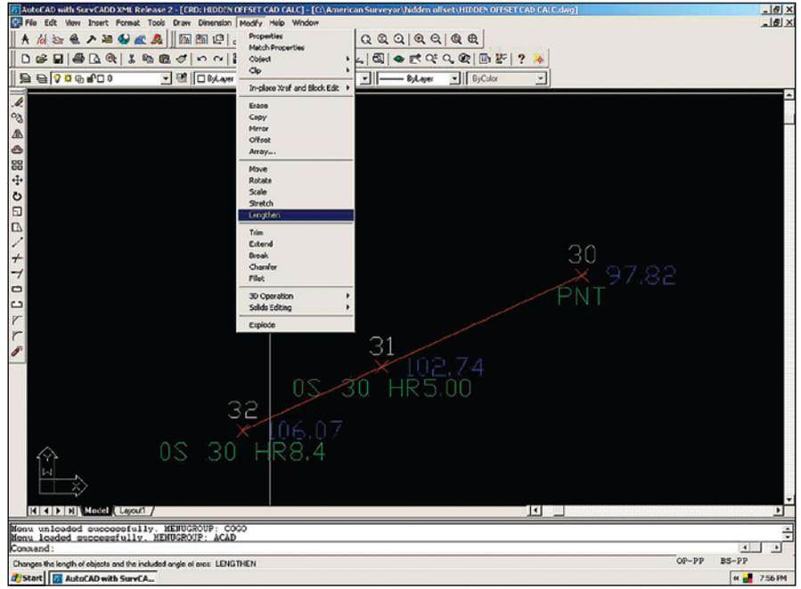
Not in for doing algebra in the sweltering heat or blistering cold? Let your CAD program do the lifting back at the office. Both IntelliCAD and AutoCAD provide a Lengthen routine that can determine the true coordinates in seconds.
