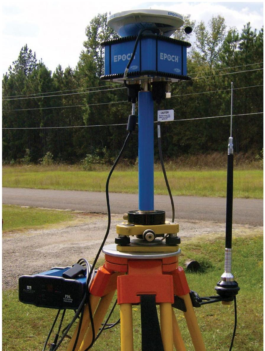
Here the Epoch 25 base station is connected to the Pacific Crest 35-watt base radio. With this combination I was able to maintain a fixed solution at the rover nearly five miles away.
