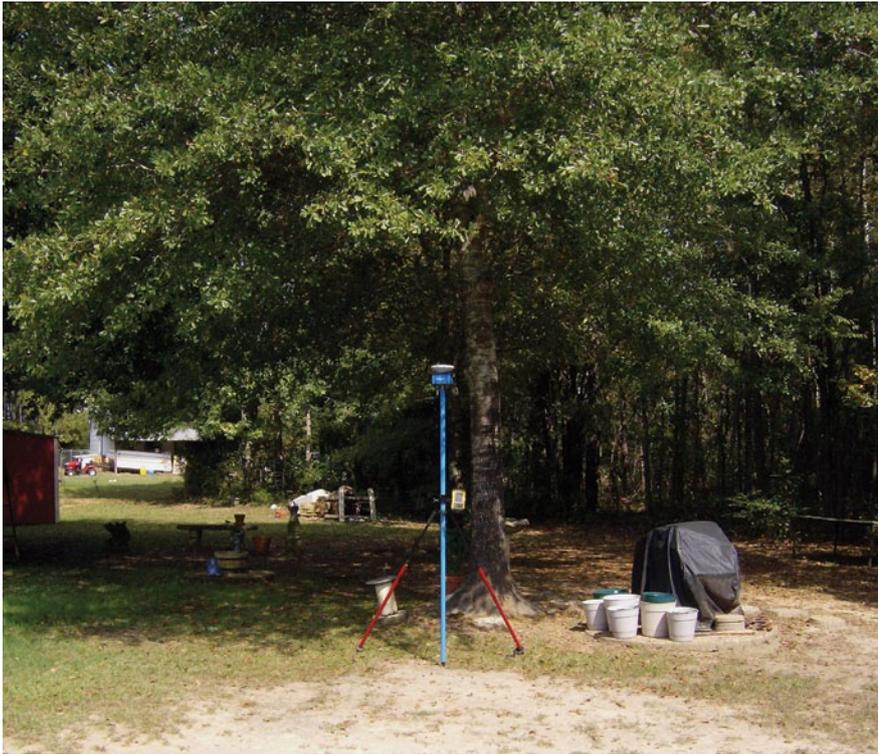
Beneath the dense canopy of this water oak tree, the EPOCH 25 was able to deliver repeatable fixed observations.
