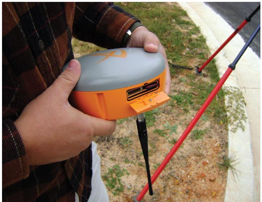
Lightweight and compact, the APS-3 allows easy access to the SIM and SD cards. The SIM card allows pick up of Internet RTK corrections; the SD card provides generous, inexpensive storage capability.
