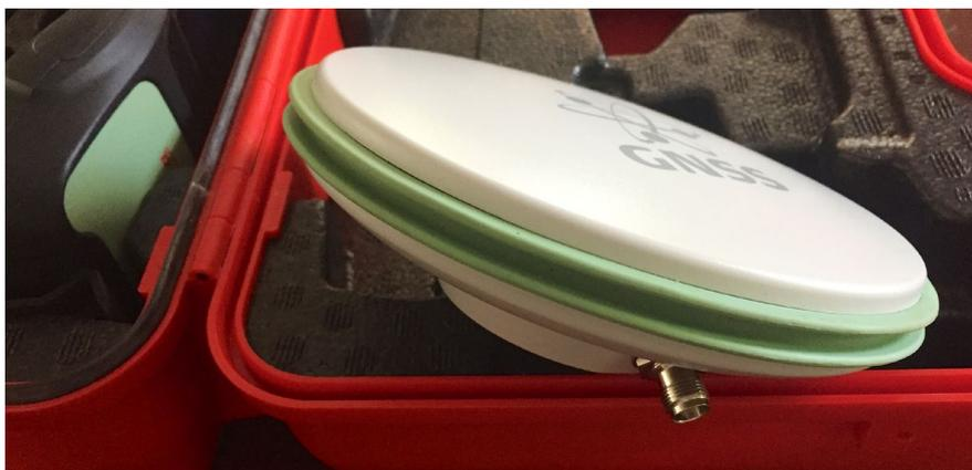
The Leica GNSS antenna is compact, having a diameter measuring less than 7-inches. It fits neatly into the hardshell case.
