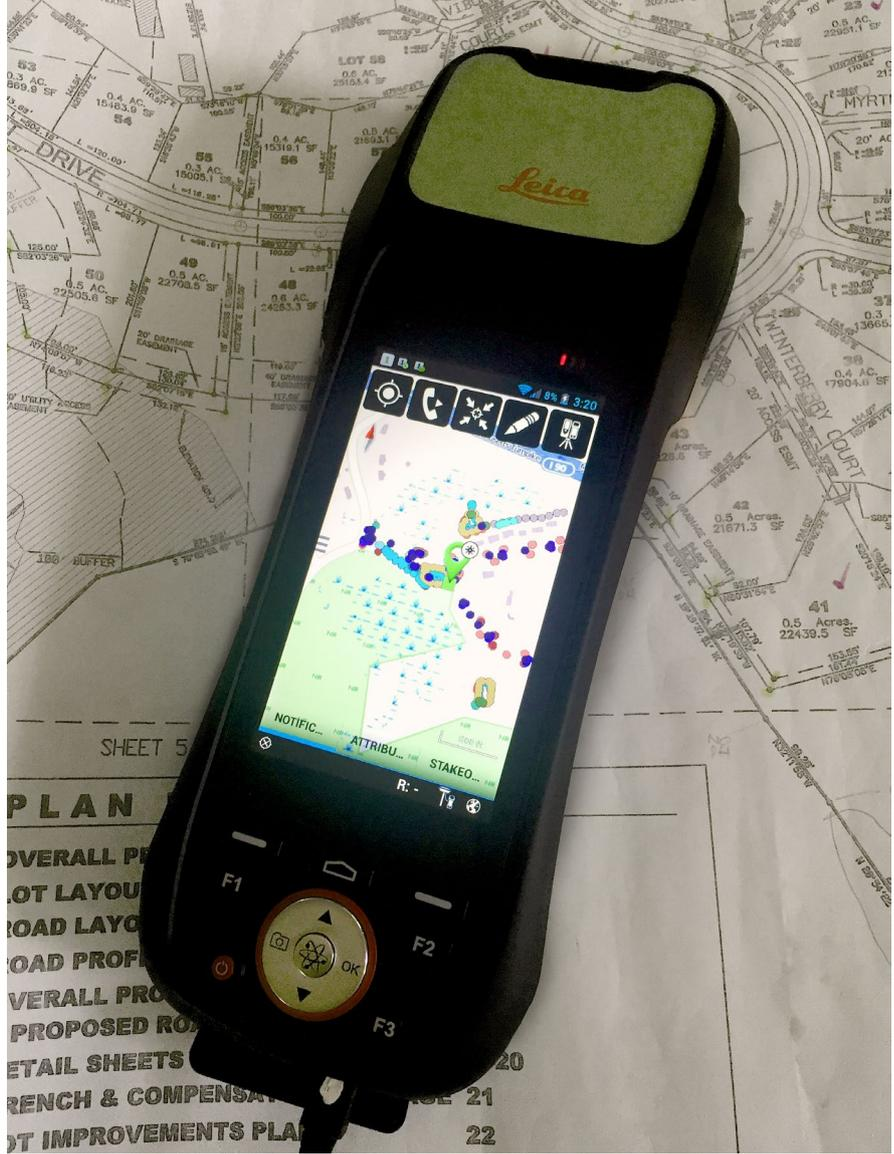
Here the Zeno displays a couple hours work within the proprietary Zeno Field software. Touch-sensitive collection options and control toggles are nicely arranged on the top.
