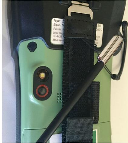
The 8 MG internal camera lens is on the rear of the Zeno to the upper left. The package includes a soft carrying handle with a built-in pouch for the stylus.
